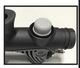
**5.** Fit the inflator bezel (p/n 15746) over the button cover (p/n 15100) and press down while rotating the bezel counter-
